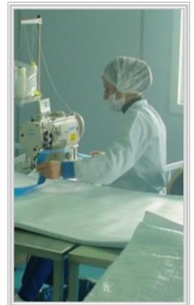
Anti-static thread is used to ensure maximum protection. All seams and webbing are sewn to the outside of the bag so no 'bits' can work free from the bag components. Glass inspection is carried out daily on windows and lights for added protection.
