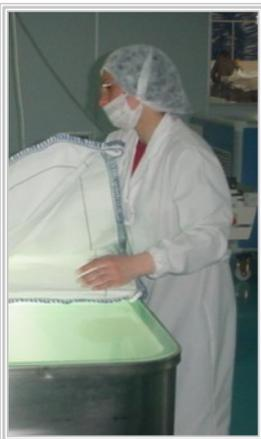
All staff working in the clean room undergo intensive training, wear shoe protection, masks, and overalls to ensure no contaminants come into contact with the bags. Air supply is monitored and controlled to ensure positive pressure at all times, A vacuum system to extract all dust is in operation 24 hours a day. The anti-static construction of the room adds to the food grade environment.
